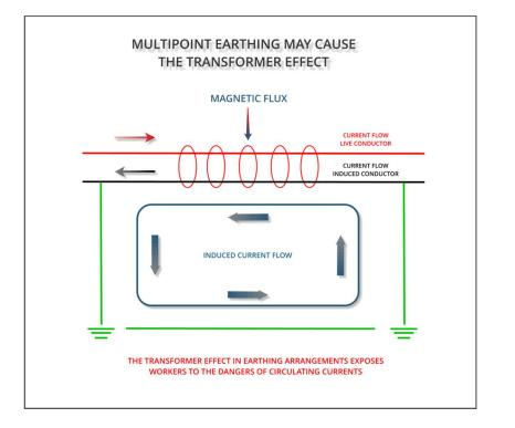
Induced voltage is caused when power lines cross over each other or run in parallel with each other and may be caused by magnetic flux or capacitive coupling. Voltages in excess of 23KV have been recorded for capacitive coupling and 1.5 KV for magnetic flux coupling. Both have caused power-line workers to be electrocuted.
