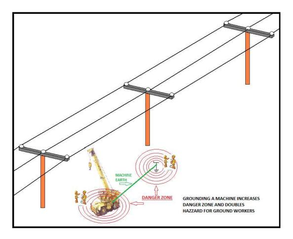
Numerous tests prove that earthing a machine does not make the worksite safe for ground workers or machine operators from the effects of Ground Rise Potential. On the contrary, earthing a machine will double the danger zone created by GRP for ground workers in the event of accidental contact with a live power line.
